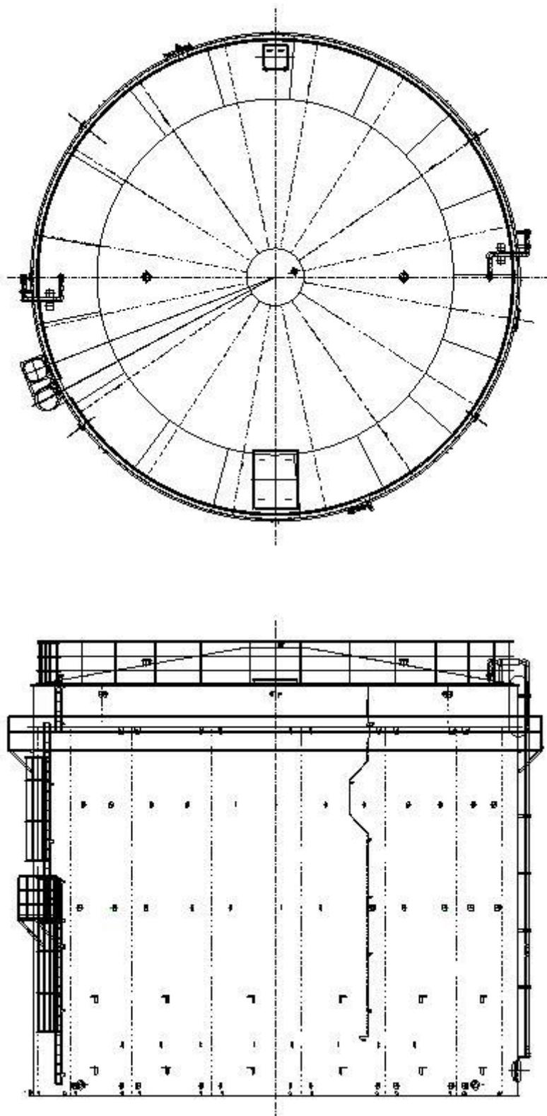
溶接型タンク概略図 (J4(2,900m<sup>3</sup>))
