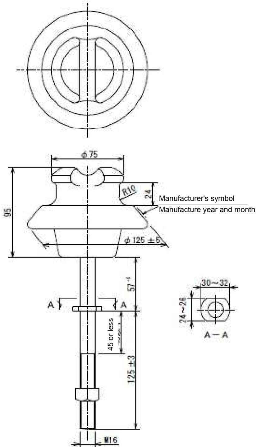
Attached figure 1: Example of an Assembled Product
