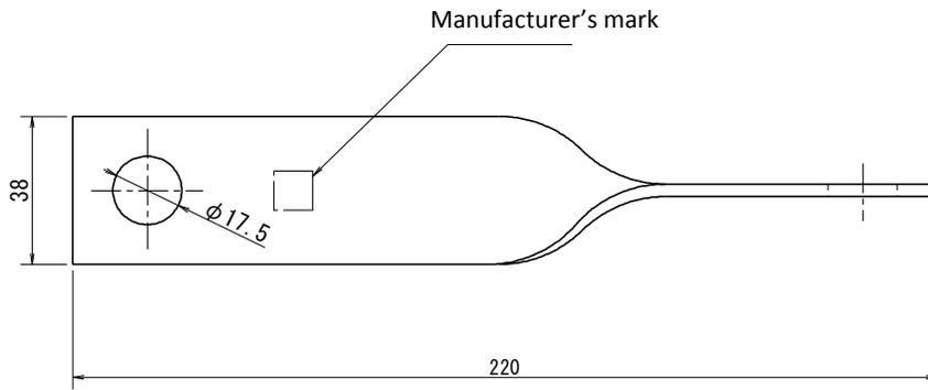
Attached figure 1: Torsion strap
