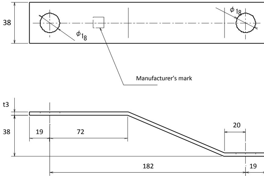
Attached figure 3: Tension strap
