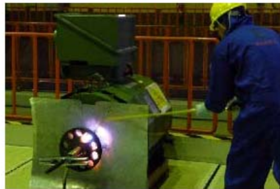
Motor Replacement training (heating operation to remove coupling)
