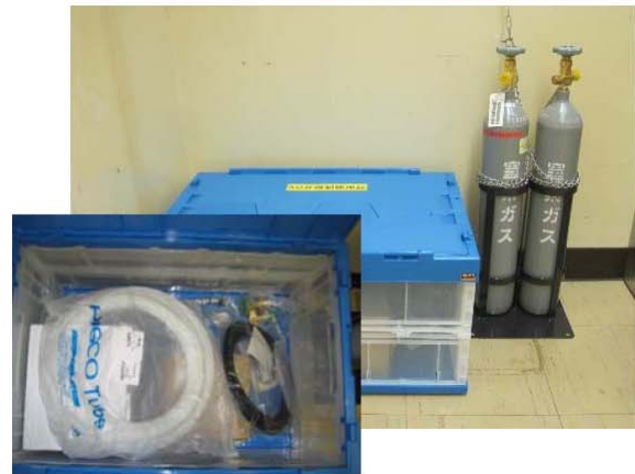
Deployment of equipment and materials for forced operation of air-operated valves (Fukushima Daiichi) (Compressed air bomb, Connection hose, connection parts etc.)
