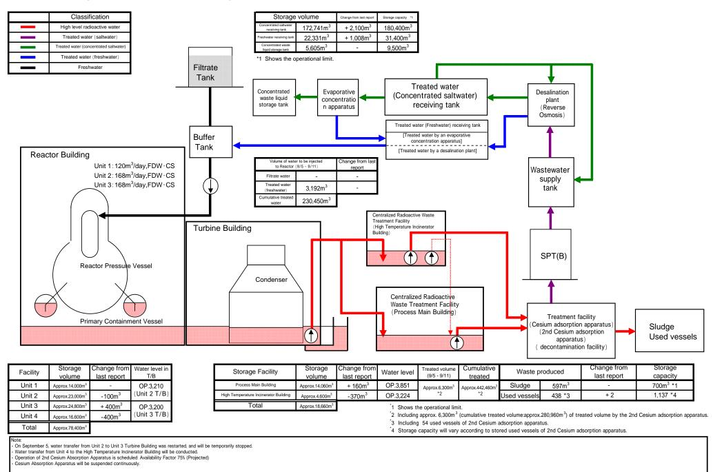
Simulation Results of Accumulated Water Treatment in Unit 1-4 T/B
