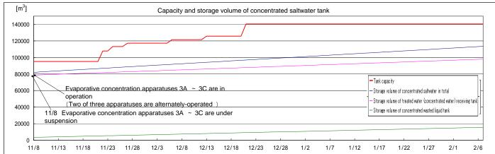
Note - Amount of water treatment is assumed to be 1,020m3/d (It can be adjusted according to level of accumulated water in T/B.)
