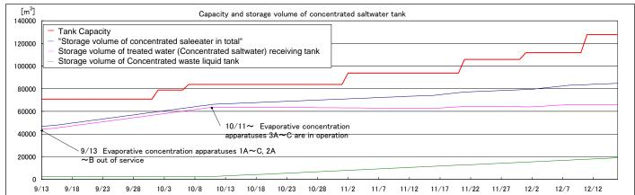
Note Assume that the handing amount by the treatment facilities is 1,140m<sup>3</sup>/d in September, 1,080m<sup>3</sup>/d in and after October. (increase the handling amount depending on the situation like the water level of accumulated water in T/B).
