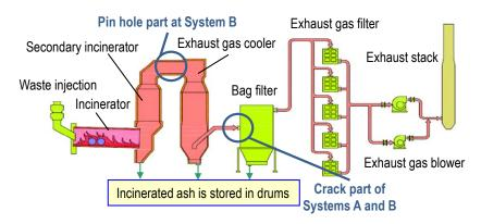
Figure 4: Overview of Radioactive Waste Incinerator
