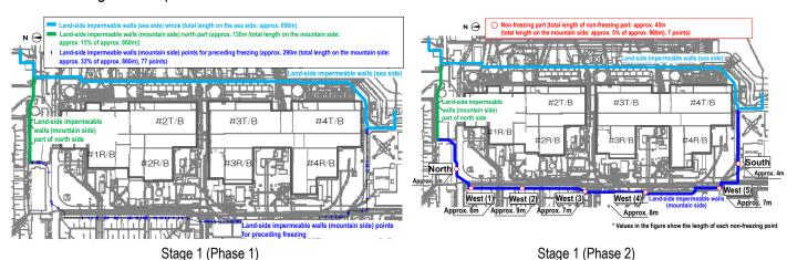
Figure 2: Scope of freezing of land-side impermeable walls
