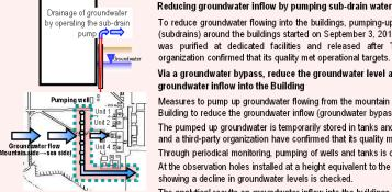
To reduce groundwater flowing into the buildings, pumping-up of groundwater from wells (subdrains) around the buildings started on September 3, 2015. Pumped-up groundwater was purified at dedicated facilities and released after TEPCO and a third-party organization confirmed that its quality met operational targets.
