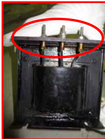
Terminal of the primary winding (Photo taken from above the transformer)
