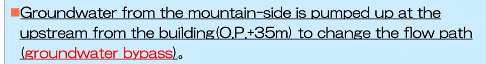
To lower the groundwater level surrounding the building (mainly the mountainside) via the groundwater bypass and mitigate the amount of groundwater inflow into the building.
