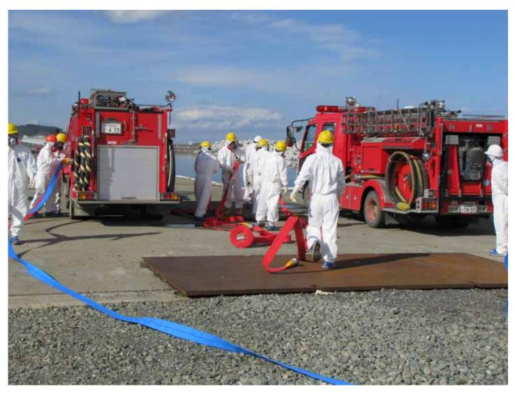
Water injection to the reactor by using pump of fire truck (at around Shallow Draft Quay) (2)
