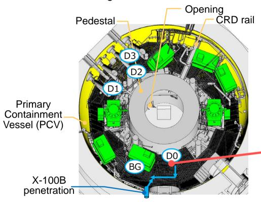
Cross section of 1st floor PCV
