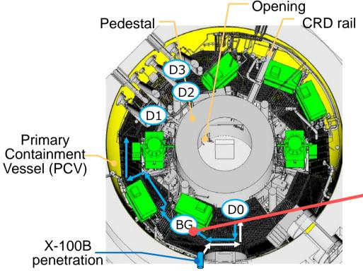
Cross section of 1st floor PCV
