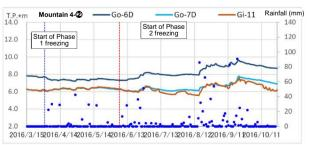
Differences in water levels inside and outside of the Landside Impermeable Wall is gradually expanding and the effects to stop water flow is observed.
