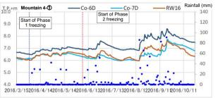
Although differences in water levels inside and outside of the Landside Impermeable Wall become stable after rainfall, it is gradually expanding and the effects to stop water flow is observed.
