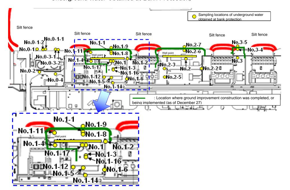
Detailed Analysis Results in the Port of Fukushima Daiichi NPS, around Discharge Channel and Bank Protection (1/12) Underground Water Obtained at Bank Protection
