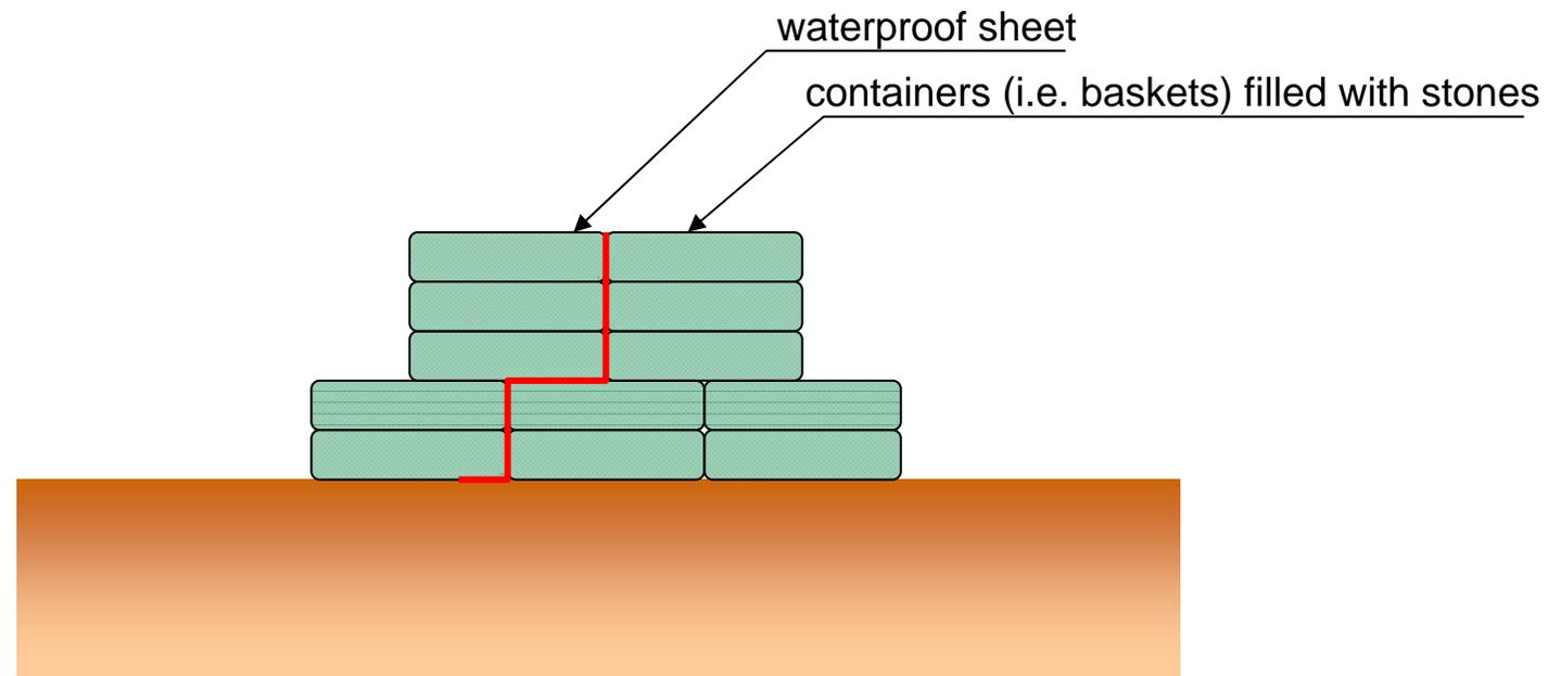
Cross Section of Temporary Seawall (Image)
