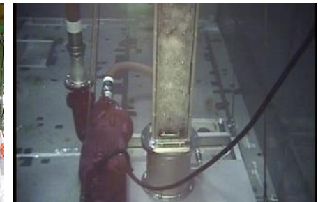
Fuel cleaning using air bubbles
