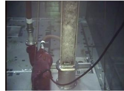
Using air bubbles to clean fuel assemblies
