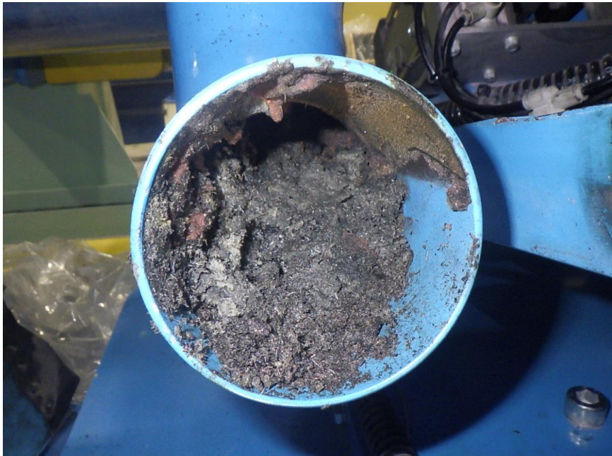
Duct with accumulated cutting scraps
