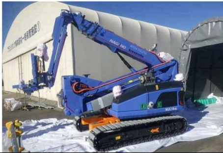
○ Elevated work platform trucks Equipped a platform to carry the \gamma imager/ FirstLook/ SPOT to each floor
