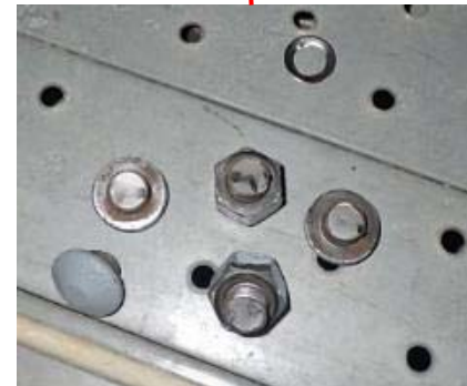
Bolts at the joint ruptured
