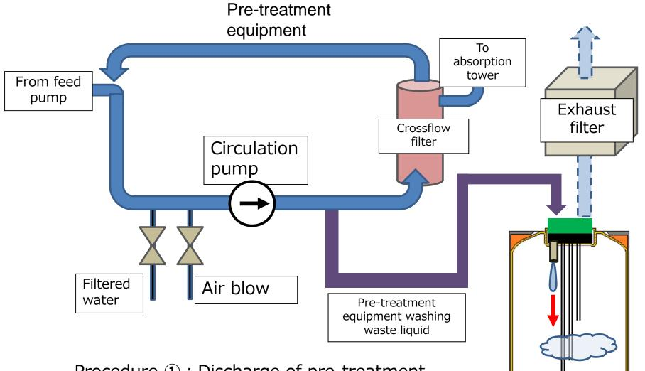
Procedure ① : Discharge of pre-treatment equipment washing waste liquid Procedure ② : Filtered water flushing Procedure ③ : Air blow
