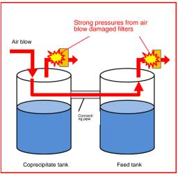
Cause of damage to coprecipitate/feed tanks (hypothesized)
