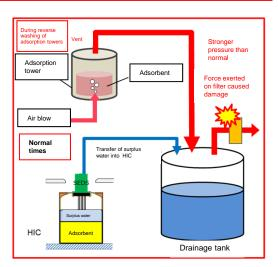
Cause of damage to drainage tank (hypothesized)
