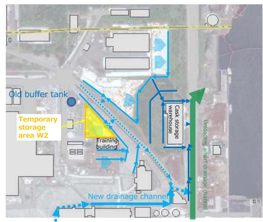
Figure 1. Locations of temporary storage area W2 and the unloading wharf drainage channel
