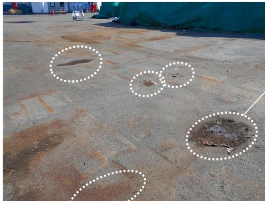
③ Stripper applied to areas where samples were taken
