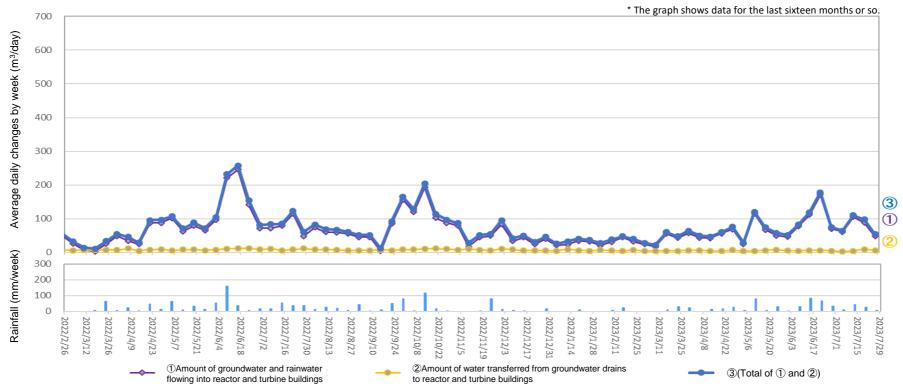
Amount of water transferred from groundwater drains to reactor and turbine buildings (From July 20, 2023 to July 26, 2023)
