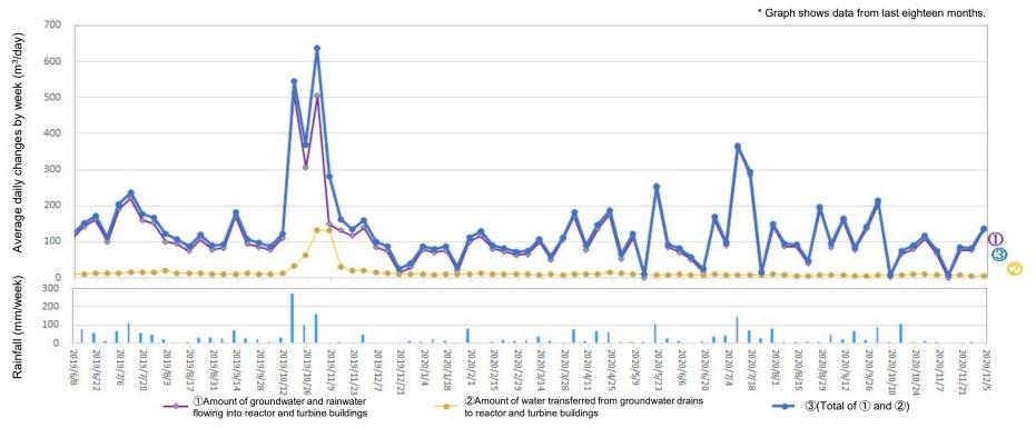
Amount of water transferred from groundwater drains to reactor and turbine buildings (From Nov 26, 2020 to Dec 2, 2020)
