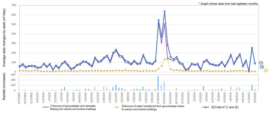
Amount of water transferred from groundwater drains to reactor and turbine buildings (From May 21, 2020 to May 27, 2020)
