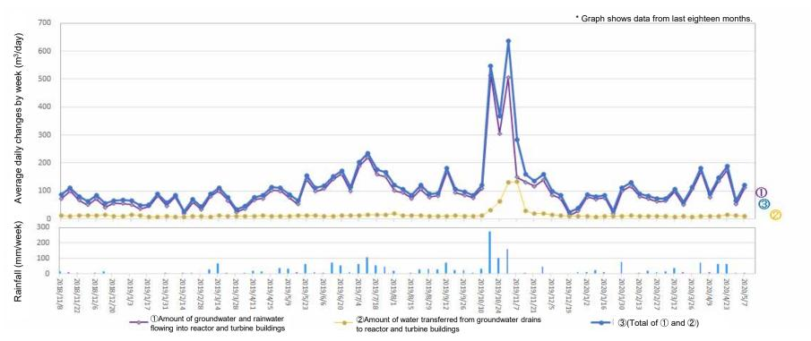
Amount of water transferred from groundwater drains to reactor and turbine buildings (From Apr 30, 2020 to May 6, 2020)
