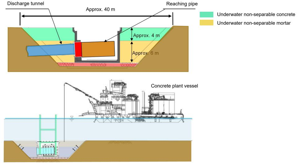
Image drawing of the backfill cross-section
