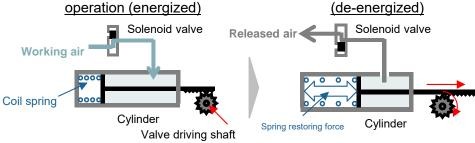
The cylinder is filled with air to maintain the valve "Open."
