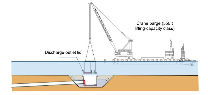
Image drawing of discharge outlet caisson lid installation
