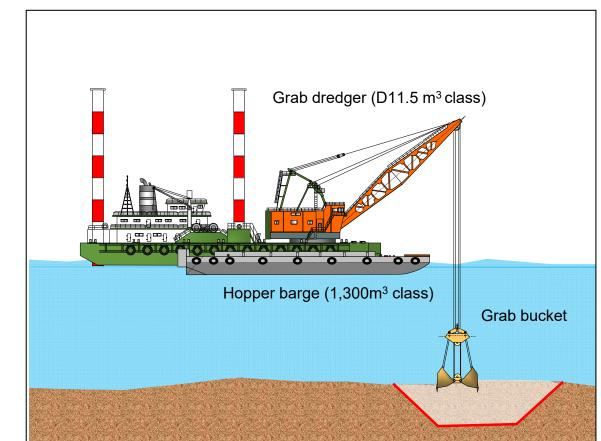
Image drawing of drilling at sea with grab dredger (sectional view)
