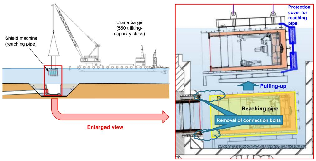
Image drawing of reaching pipe (shield machine) removal
