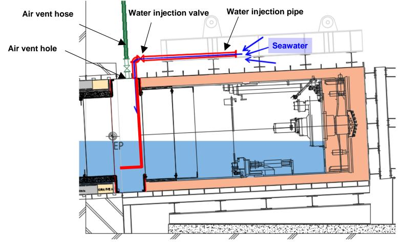
Image drawing of water injection work condition
