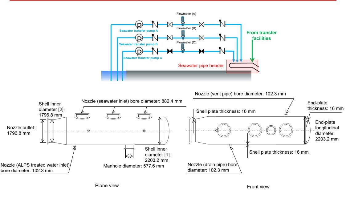
Structural drawing of seawater pipe header
