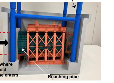
Lateral view of discharge outlet caisson
