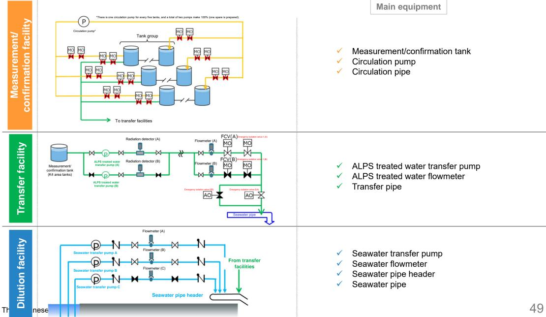
2-1(1) [5] Structure and strength of equipment, protection against natural phenomena such as earthquakes and tsunamis TEPCO [3]-2 Basic specifications and main structure of the measurement/confirmation tank
