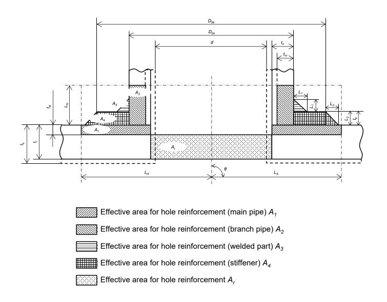
Diagram of calculation for hole reinforcement
