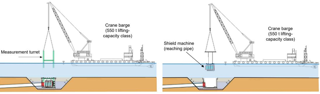
Image drawing of measurement turret removal
