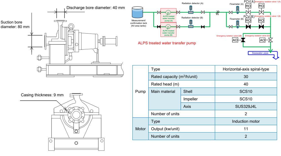
Structural drawing of ALPS treated water transfer pump The Japanese version shall prevail. 2-1(1) [5] Structure and strength of equipment, protection against natural phenomena such as earthquakes and tsunamis [3]-5. Basic specifications of ALPS treated water flowmeter and seawater flowmeter **TEPCO**
