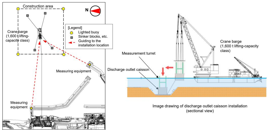
Image drawing of discharge outlet caisson installation The Japanese version shall prevail view) τΞρςο
