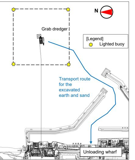
Image drawing of drilling at sea with grab dredger (plane view) The Japanese version shall prevail.
