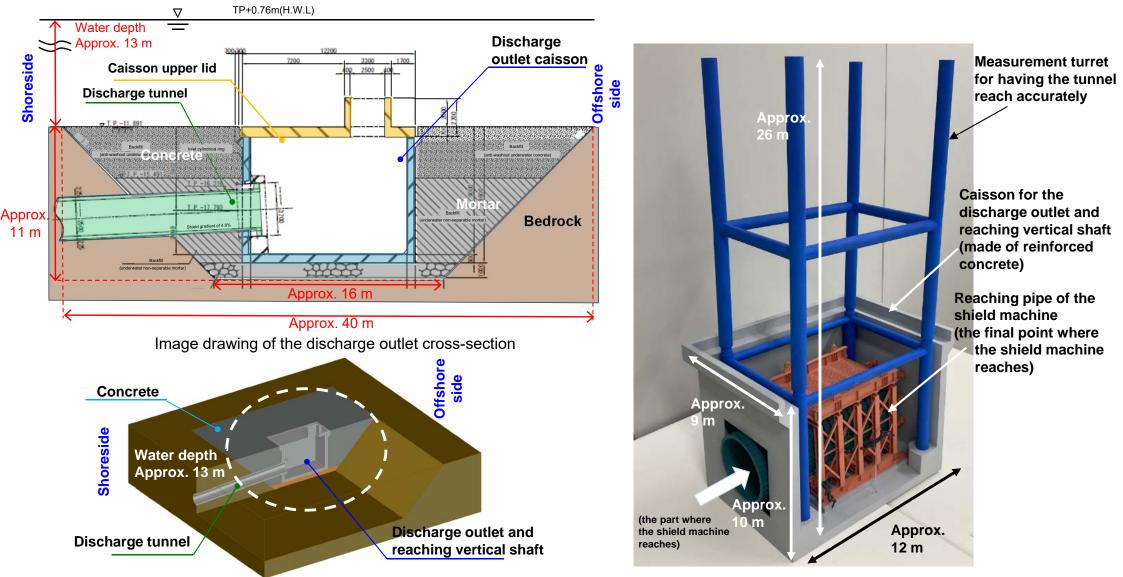
Image drawing of discharge outlet
