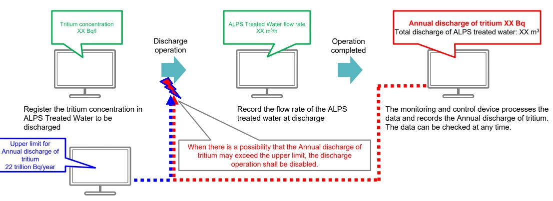
Set the upper limit for the annual release on the monitoring and control device beforehand.
