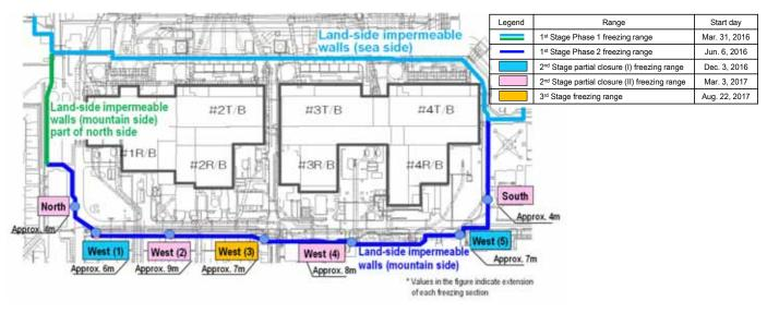
Figure 3: Closure parts of the land-side impermeable walls (on the mountain side)
