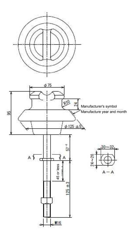
Attached figure 1: Example of an Assembled Product
