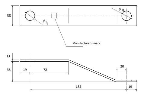
Attached figure 3: Tension strap
