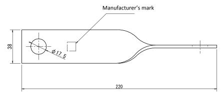
Attached figure 1: Torsion strap
