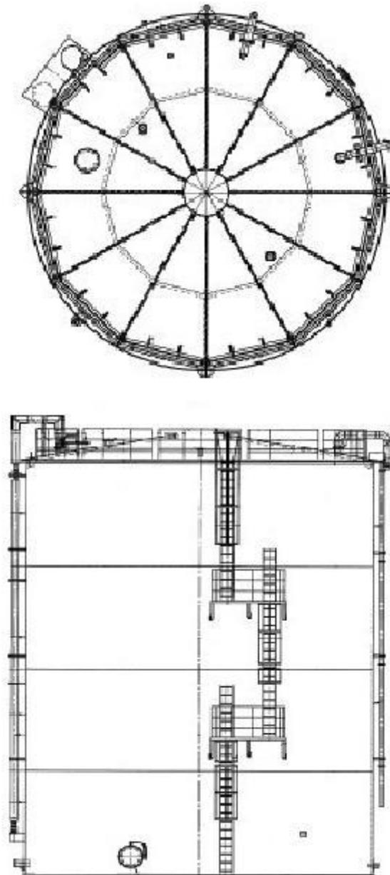
溶接型タンク概略図 (G1 南 (1,330m<sup>3</sup>))
