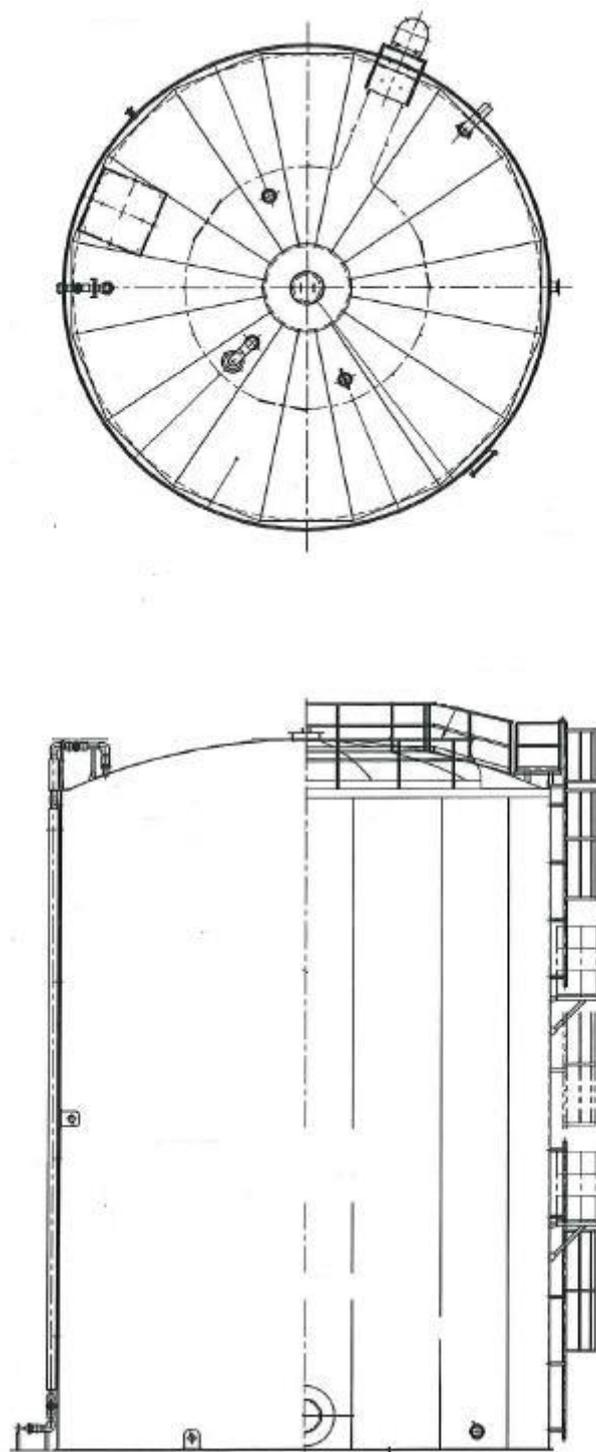
溶接型タンク概略図 (B, B 南(1,330m<sup>3</sup>))
