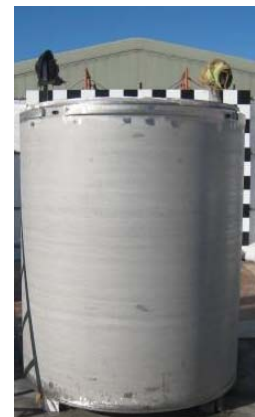
(HIC補強体外観)
